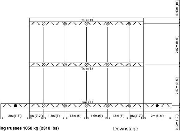
Maximum load bearing capacity of all 3 bearing trusses 1050 kg (2310 lbs)
