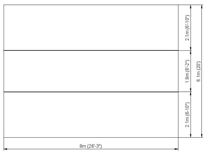
Downstage Capacity: 100 lbs/ft<sup>2</sup> (5 kN/m<sup>2</sup>)
